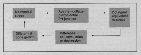
This simple block diagram illustrates the control system which regulates the growth of bone in response to mechanical stress (short of failure) in all mammals, as postulated by the author. The
