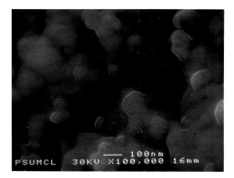
Figure 1. Scanning electron micrograph of the silver deposit on a single nylon fiber. The silver deposit is composed of small units averaging 100 nm which appear to be made of a number of single crystals. Crystal angles can be seen on the edges of individual deposits. Magnification indicated by the scale bar.
